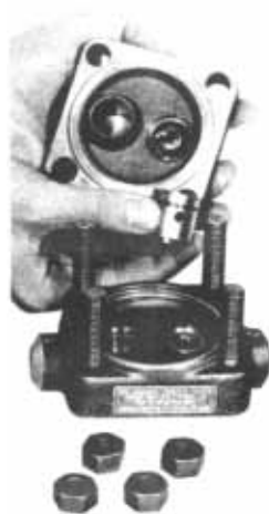
Figure 4—Seat removed to show valve and control cylinder.
